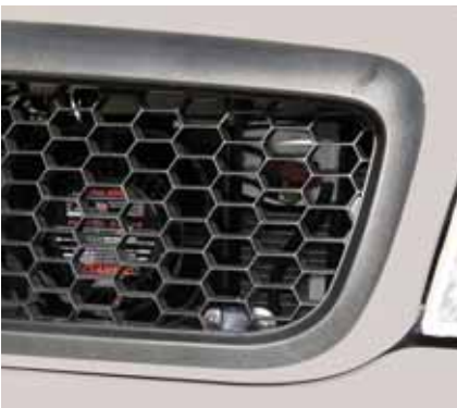
SA315P with vehicle specific mounting in grille of Crown Victoria.
