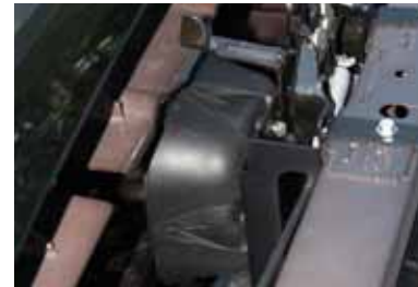
Photo shows mounting placement of SA315P between grille and radiator.
